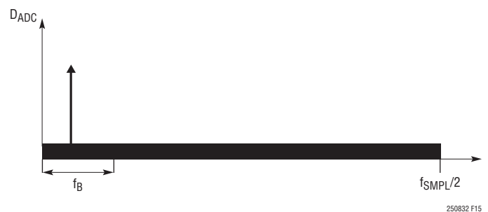
Figure 15. Frequency Spectrum of SAR ADC Core Output
